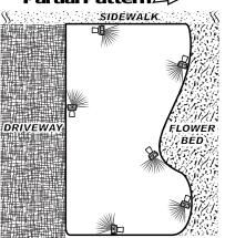
Maintain a consistent walking speed of 2 to 3 mph or the spread width and application rate will change.
